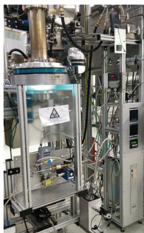
Figure 1. Left: Reactive zone of the microwave plasma reactor at the University Duisburg-Essen. Right: Few-layer graphene as seen under the transmission electron microscopy.
