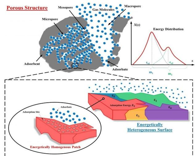
Fig. 2. Adsorption on a surface with different energy sites
