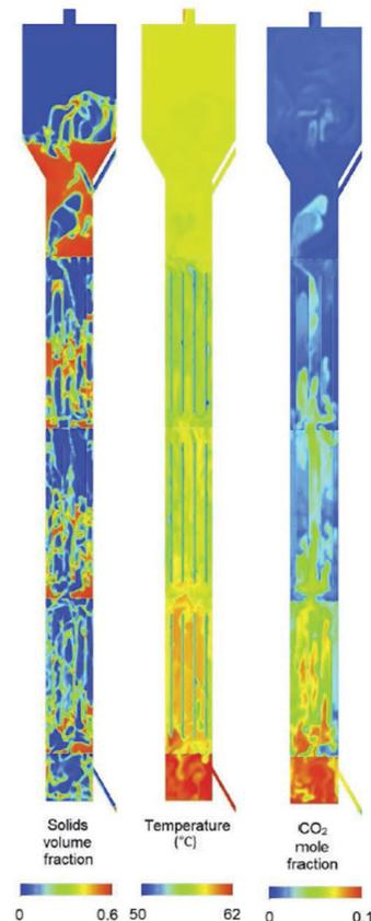
Figure 1: An example of a TFM simulation of a fluidized bed CO<sub>2</sub> adsorption reactor with particle-wall heat transfer included
