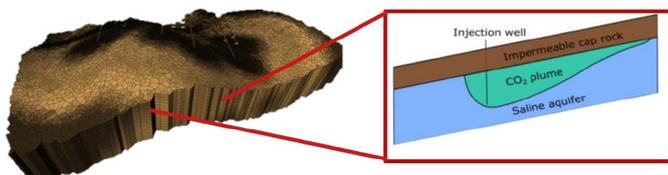
Figure 1: Subsurface CO<sub>2</sub> storage
