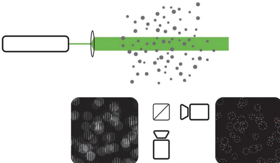
To characterize the spray, we will use a thick laser sheet and a 2-camera setup that measures both the particle-size and the distribution of fluorescent nanoparticles. IPI image adapted from Evans *et al.* Rev. Sci. Instrum. **86**, 023709 (2015)
