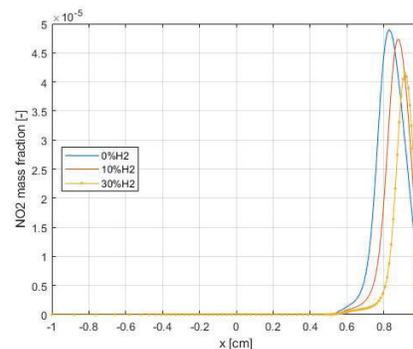
Fig 2: The NO<sub>x</sub> profile of 1-D NH<sub>3</sub>/H<sub>2</sub> diffusion flame
