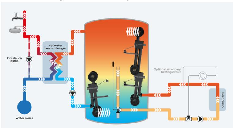
Both for the performance of the overall system, as well as its efficiency, careful attention to stratification is warranted [1]. To this end, the design of the diffusers used on the inlets deserves particular attention, to prevent inflow disruption of the thermal layering.
