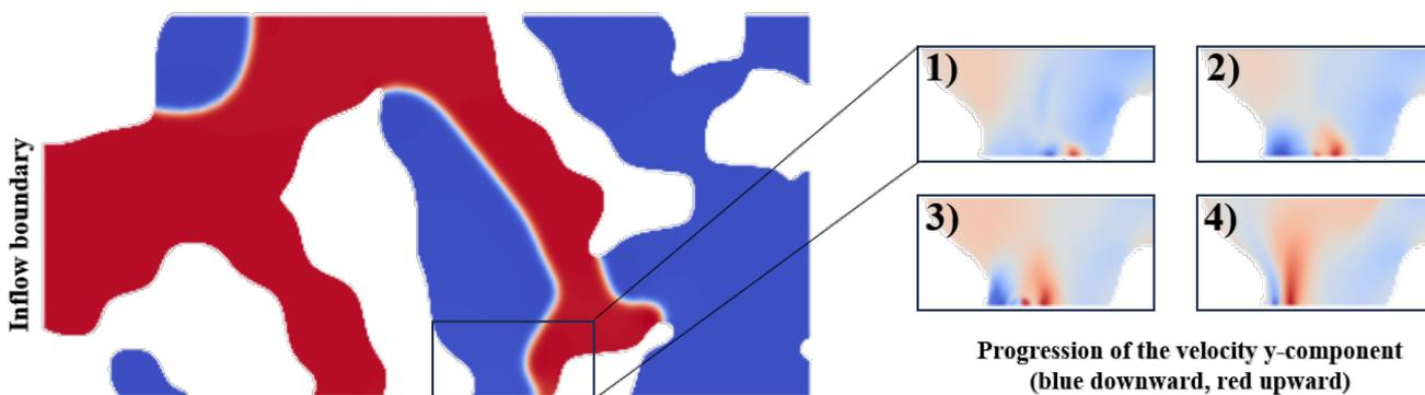
**Fig 1.: Multi-phase flow through porous medium. Left: phasefield of two constituents at the time that an outflow boundary is reached. Right: evolution of the velocity field at what should be the outflow boundary. Showing erroneous and unstable velocity inflow (backflow) spikes.**
