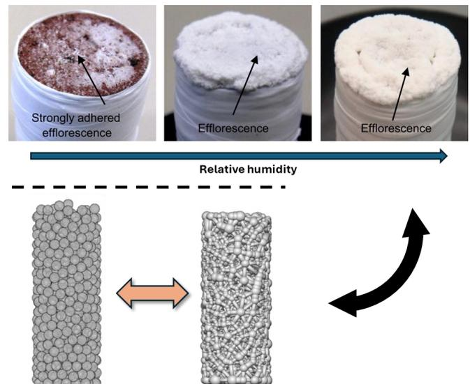
The quality of the salt deposition is heavily influenced by the drying condition. You will investigate this fascinating phenomena via pore network modeling and experimental tools. Images taken from [1] and [3]
