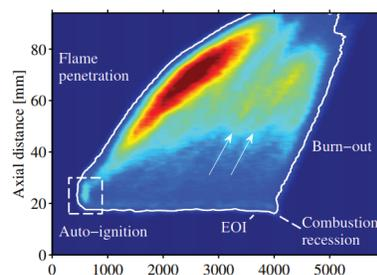
Figure 2. Radially integrated OH\* intensity obtained in the EHPC as a function of axial distance and time, with a contour defined by the intensity at the location of the steady flame lift-off length.
