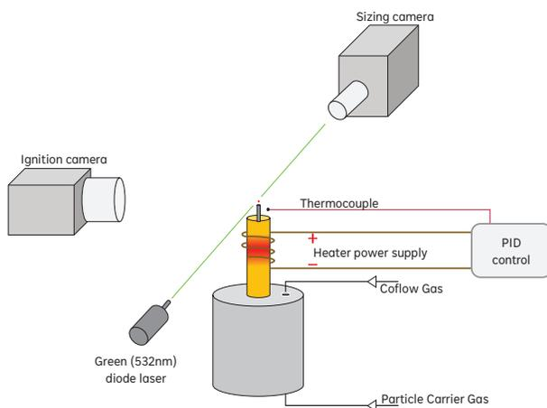
Fig. 1 Schematic diagram of the single particle burner experiment setup.
