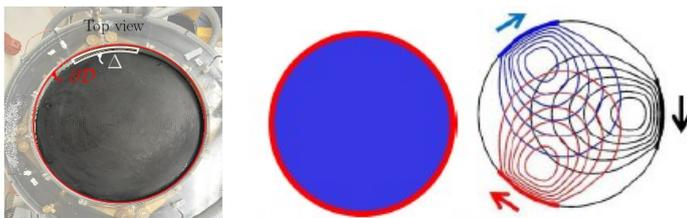
(a) Boosting heat transfer by stirring. (b) Case study: heating of a cold (blue) fluid by wall-driven stirring.
