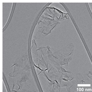
Figure 1. Left: Reactive zone of the microwave plasma reactor at the University Duisburg-Essen. Right: Few-layer graphene as seen under the transmission electron microscopy.
