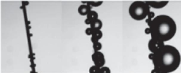
Hydrogen bubble formation on a gold wire. As long as they are attached to the wire, they reduce its effective surface area. (Figure from Chen et al. (2018) JPC C122: 15421.)
