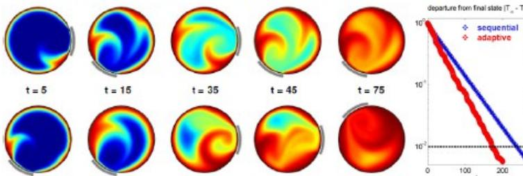
(c) Flow-enhanced heating driven by sequential (top) vs. adaptive (bottom) wall actuation. (d) Heating rate.
