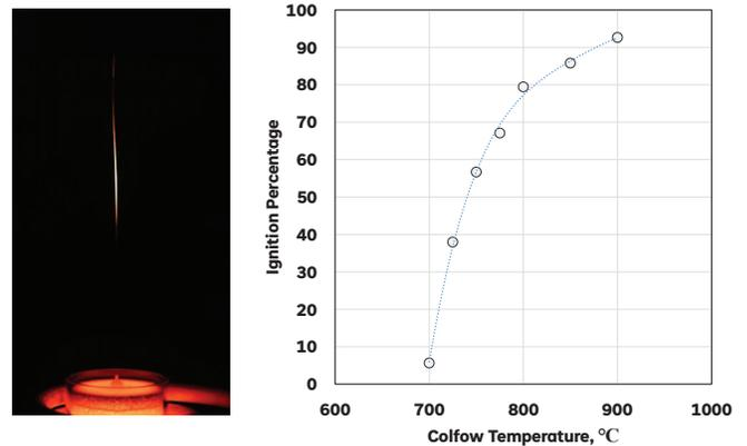
Fig. 2 Burning iron particle by hot coflow (left) and Ignition percentage of 45-53  $\mu\text{m}$  iron particles (right).
