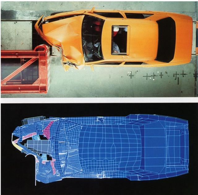
Fig 1: Crash-test simulation. Credit: Cray Research Inc.
