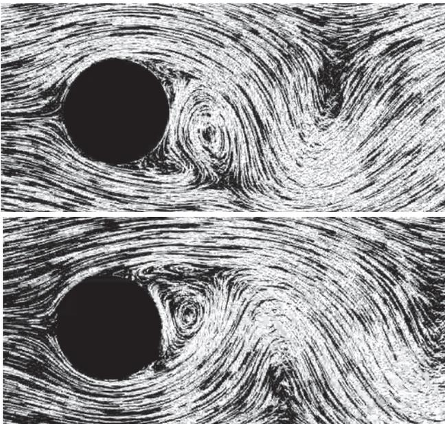
**Fig 1:** RANS simulation with clear low-frequency oscillation components.
