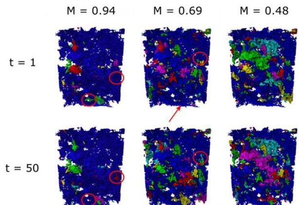
Figure 2: The distribution of the oil phase (rock and water transparent) for different viscosity ratios ( $M$ ) at two different times  $t$ . Each connect region of oil has been assigned a different colour to show the connectivity.
