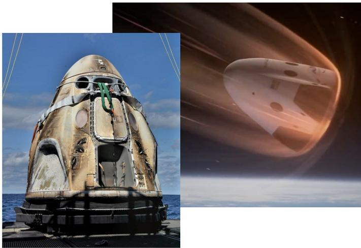
*Scorched heat shields after successful reentry of the SpaceX Dragon (left) and artist's impression of reentry flight (right)*
