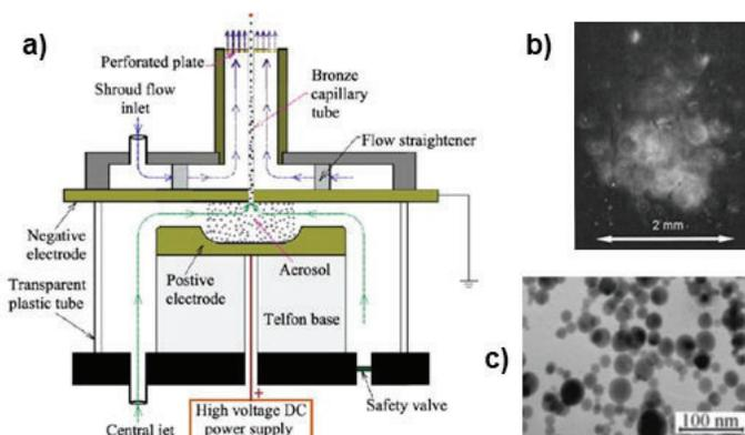
Fig 1. a) Schematic micro-burner with electrodynamic dispersion system for metal aerosol combustion. b) A short-exposure image of Al aerosol flame showing nano-particle clouds around burning Al particles. c)  $Al_2O_3$  nano-particles generated by the flame.
