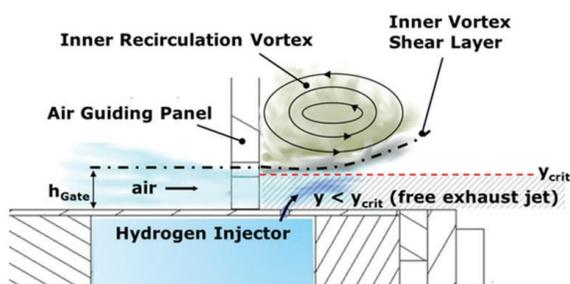
Fig 1: Micro-mix injection, drawn by Funke [1]
