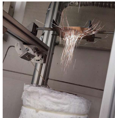
Figure 2: An experiment performed by the previous master student. Iron particles are combusted before colliding with a metal plate to simulate deposition on a reactor surface.
