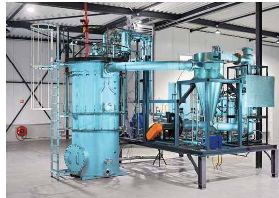
Fig. 2. 500 kW iron powder combustion system operated at Metalot
