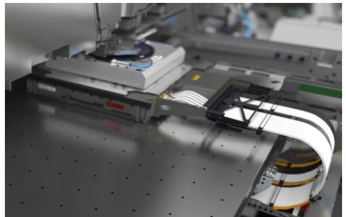
Fig 1a: Hoses in high precision motion stage (courtesy: ASML)
