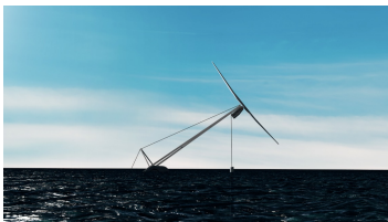
Figure 1: TouchWind rotor during normal operating conditions.
