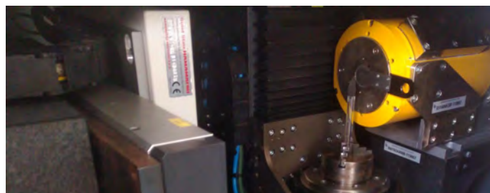
Fig. 1. Micro computed tomography equipment in the multi-scale lab.
