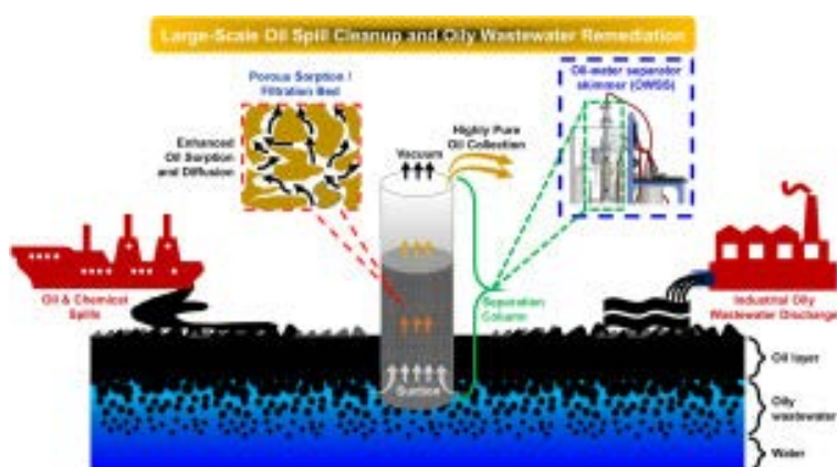
Fig. 1. Filtration of contaminated water by sponges [1]
