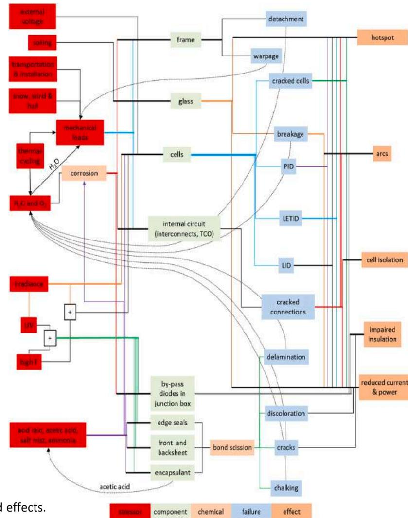
Flow diagram representing the relationships between stressors, components, failures and effects.
