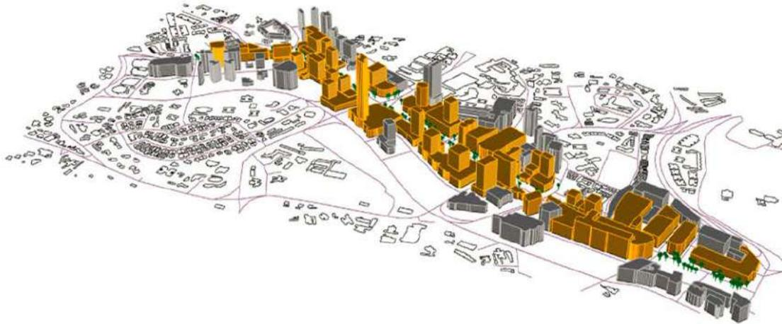
Given a specific built environment with objects such as buildings and vegetation, the available annual solar irradiance on surfaces such as roofs and facades and the visual impact of these surfaces determines the potential for PV applications.
