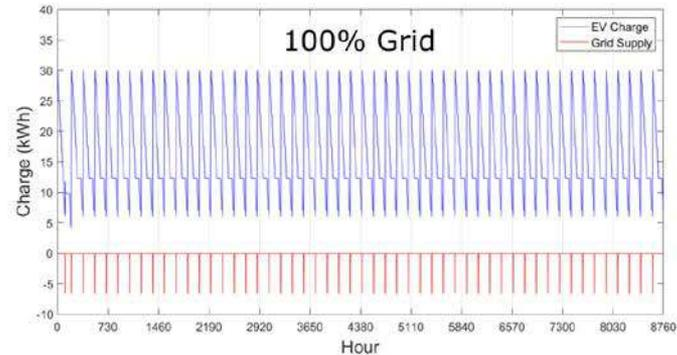
EV charging by PV charging station (blue) and grid (red) in each scenario for the system located in the Netherlands (with 10 kWh BESS). Clockwise from top left: 100% PV ( $A_{PV} = 5$  kWp), 75% PV + 25% Grid ( $A_{PV} = 1.2$  kWp), 100% Grid, 50% PV + 50% Grid ( $A_{PV} = 0.8$  kWp).
