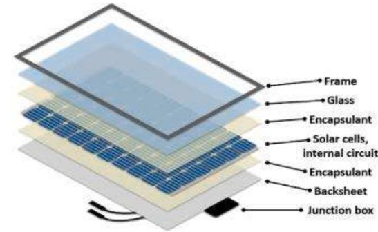
common configuration of cadmium telluride PV modules
