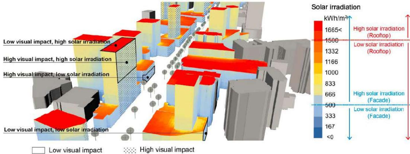
Visualisation results of a simulation of 3D annual solar irradiation for Orchard Street in Singapore showing different annual irradiation levels and classes of visual impact. Figure from Sun et al. , 2021.
