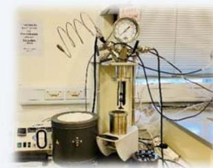
**Bench-scale Hydrothermal Reactor**
