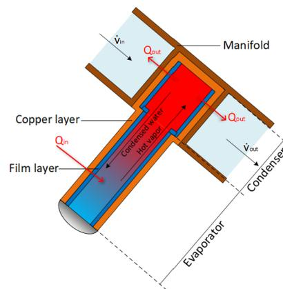
Liquid flows through the inside of the manifold to transfer heat from the manifold to the storage tank, and the heat transfer inside the manifold is a critical factor, as well as the operation of the heat pipe during the highly transient multi-pass operation.
